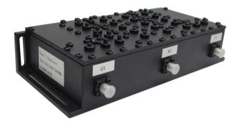
This is a cavity duplexer for 2600 MHz UMTS / LTE Band 7 operation.
